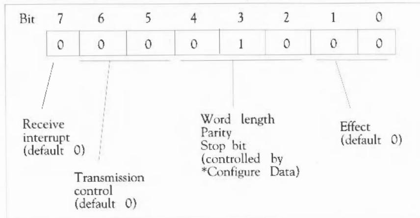
The eight-bit number in the above diagram corresponds to \*FX 156, 16. This sets the read/write asynchronous communications state to 8 bits, no parity, two stop bits. It sets RTS low and disables transmit and receive interrupts. This setting will work for many models of serial printer.
