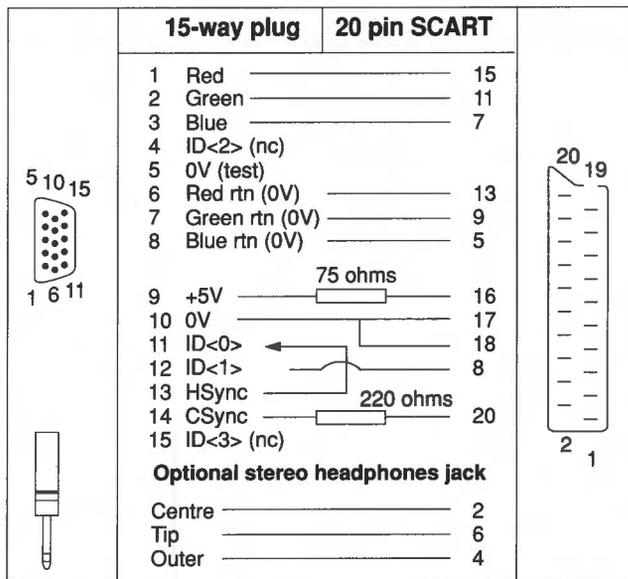
**Note 1:** HSync (pin 13) linked back to ID<0> (pin 11) tells the computer that composite (rather than vertical) sync is required, and that only modes compatible with a TV standard monitor can be displayed.
