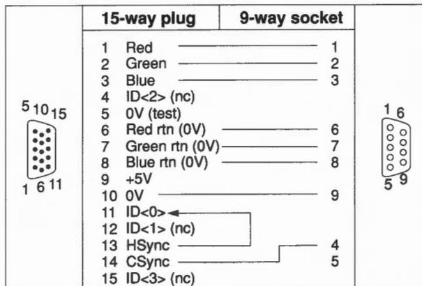
**Note:** HSync (pin 13) linked back into ID<0> (pin 11) tells the computer that composite (rather than separate) sync is required, and that only modes compatible with a TV standard monitor can be displayed.
