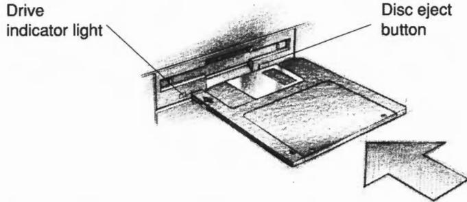
The disc clicks into place when it is fully inserted.
