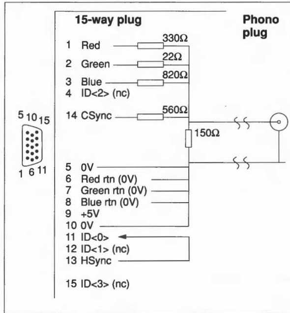
**Note:** HSync (pin 13) linked back into ID<0> (pin 11) tells the computer that Composite sync (CSync) is required rather than VSync on pin 14 and that only modes compatible with a TV standard monitor can be displayed.
