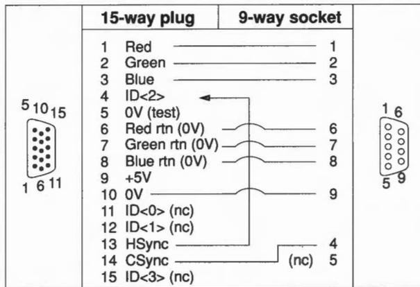
**Note:** HSync (pin 13) linked back into ID<2> (pin 4) tells the computer that composite (rather than separate) sync is required, and that modes compatible with a Multiscan monitor can be displayed.
