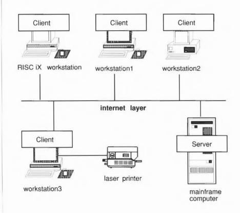
On a typical network, a server would be a mainframe computer with a lot of disc storage and a large amount of memory. The sample network used in this chapter shows a typical set-up.
