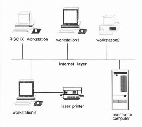
The machines communicate using the internet protocols layer over a combination of ethernet, cheapernet and Econet cables.
