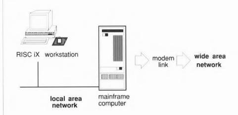
In this example, the mainframe acts as a gateway between the two networks, by being able to transfer the information from one type of network and communication line to another type of network and communication line.
