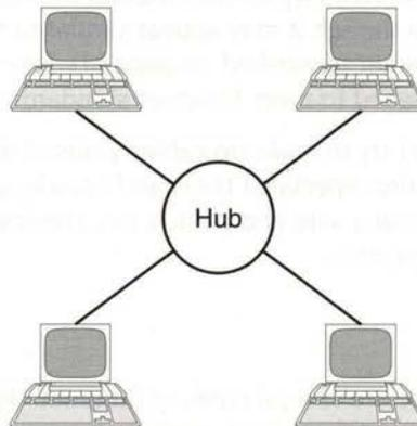
Figure 6.2 Star topology, as used by twisted-pair Ethernet
