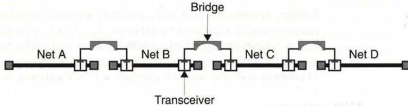
Figure 7.4 A network without a backbone
