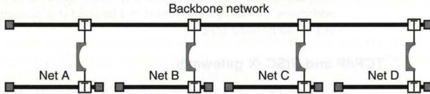
Figure 7.5 A network with a backbone
