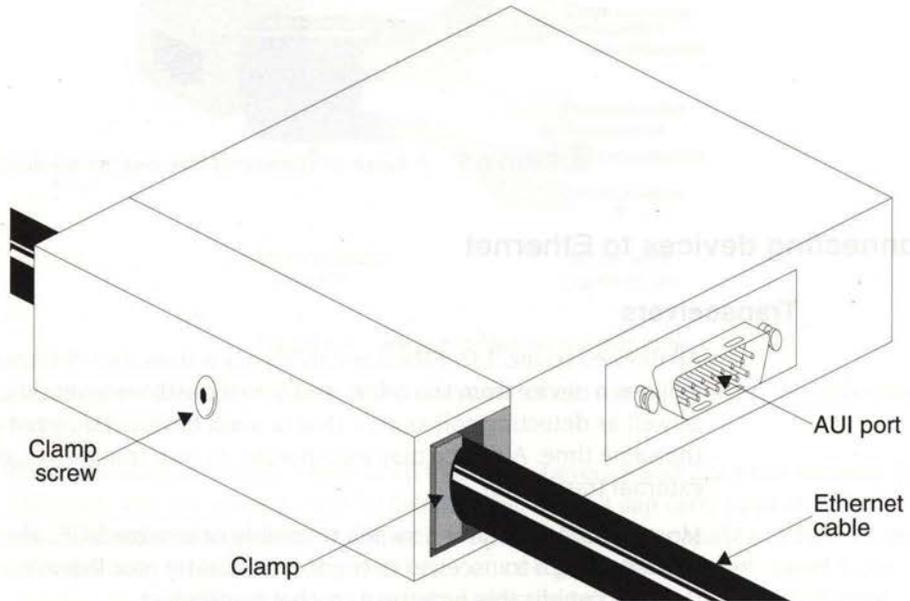
Figure 6.6 A thick Ethernet transceiver
