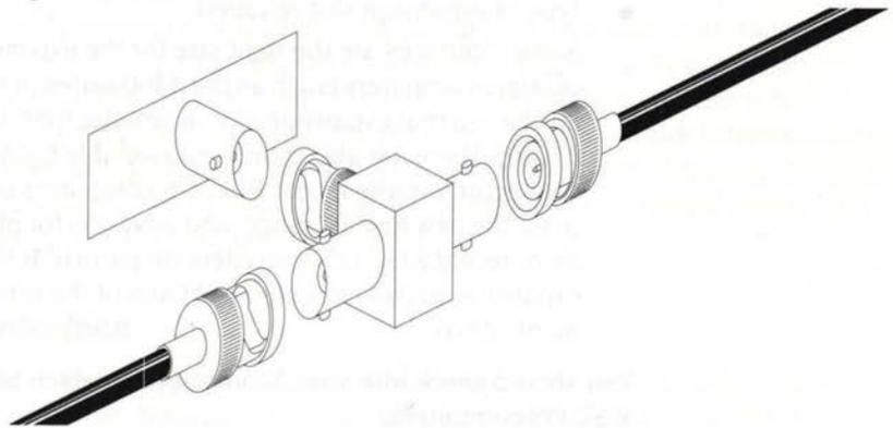
Figure 6.8 A BNC connector, T-piece and cabling
