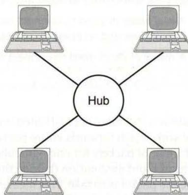
Figure 7.3 A hub with stations connected via twisted-pair Ethernet
