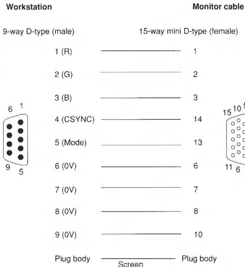
Alternatively, you can make a single cable to connect from the workstation to the monitor without an adaptor.
