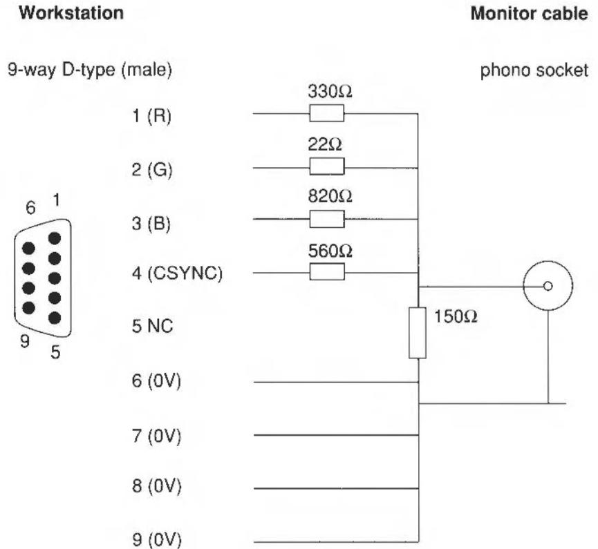
Alternatively, you can make a single cable, which connects directly from the workstation to the monitor. It requires the same mixing resistor network. If you are unsure about how to make either of these, then contact your supplier.
