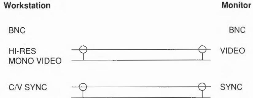
For monitors using three type ME cables, the connections are as follows:
