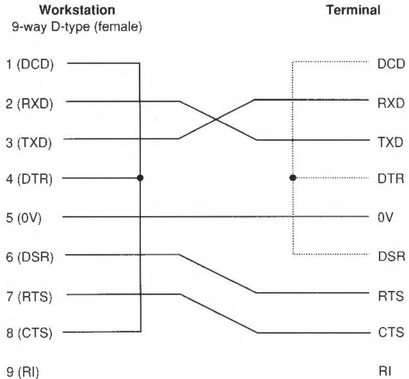
An important point to note is that the terminal monitors the status of the lines DSR (data set ready) and DCD (data carrier detect). It also raises and lowers DTR (data terminal ready) as appropriate. In many cases, where 'modem control' is not required (which is the case with most terminals) it is appropriate to strap all these lines together, and thus only use the three lines of transmitted data, received data and common return.
