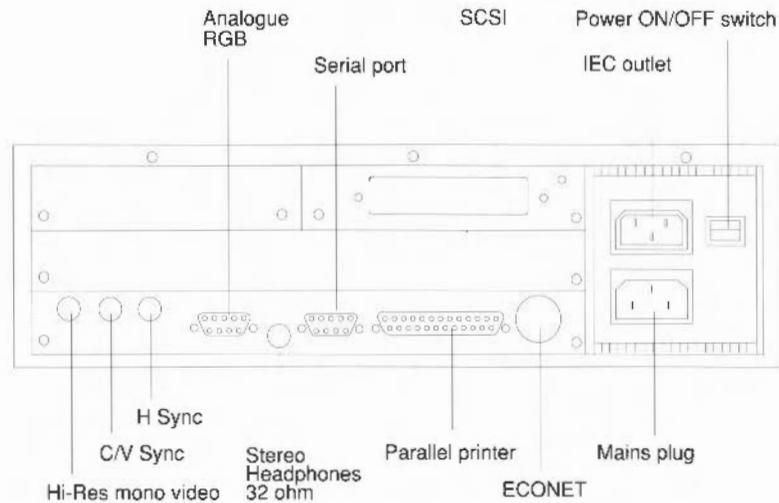
The following subsections describe the connectors on the back of the computer:
