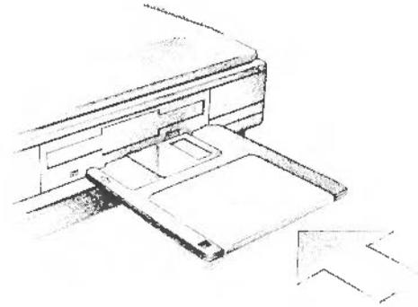
The disc clicks into place when it is fully inserted.
